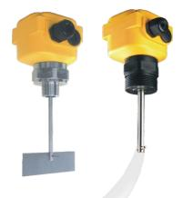
Ambient Operating Temperature -20...80°C SPDT Max. 250VAC 3A Contact Output 200°C and 450°C High Temperature Option Optional Aluminum Head Option Dustproof Special Shaft for Optional Sealing Adjustable Torque Small and Compact Design for Simple Assembly Stainless Steel Mechanical Parts and Robust Gear Engine Maintenance Free Easy setup Suitable for Detecting Very Light Particulate Solids Screw Thread
